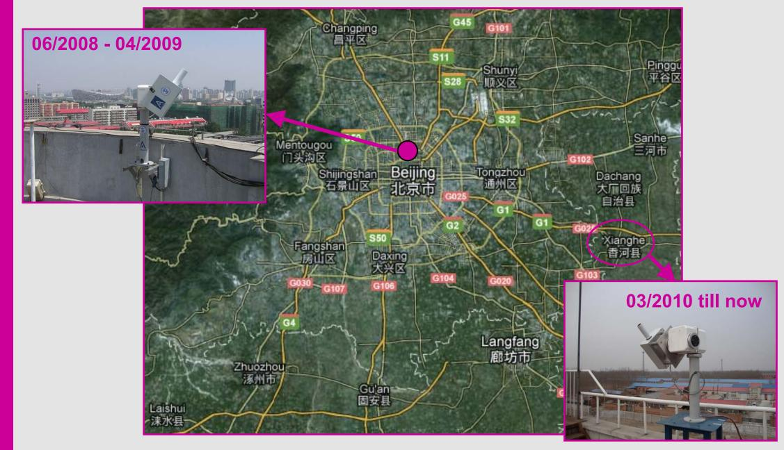
The instrument measures sunlight scattered at different elevation angles (2°, 4°, 6°, 8°, 10°, 12°, 15°, 30°, zenith) towards the horizon (~15 minutes per scan)
