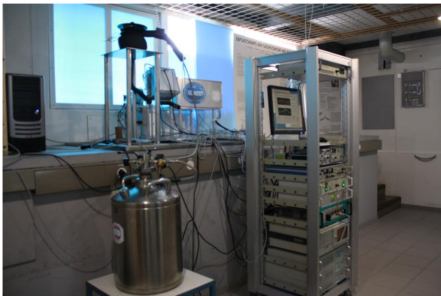
Figure 15. A typical ozone microwave radiometer (GROMOS at Bern)
