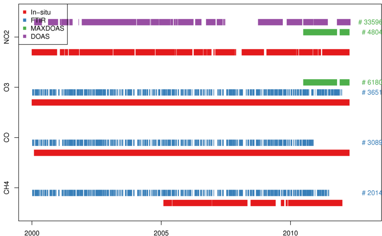
Figure 1: Data availability for the site JFJ. The on the right indicate the number of collocated data from in-situ observations for each remote sensing device. The collocation criterion was simply the availability of in-situ data with a window of 6 and 2 hours around the remote sensing data for FTIR and MAXDOAS/DOAS, respectively.
