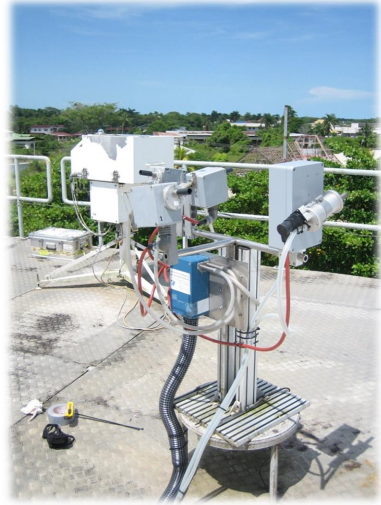
The MAX-DOAS telescope unit in Paramaribo, Suriname
